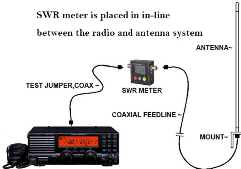
**Correctly use the radio to measure S.W.R.**
